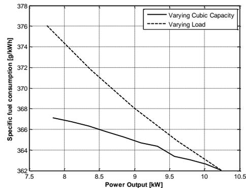
Figure 23. Specific fuel consumption by indicated power.
