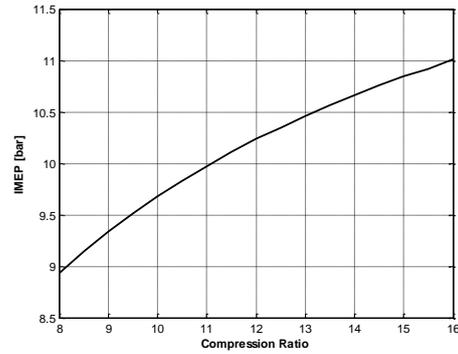
Figure 8. Influence of the compression ratio on the IMEP
