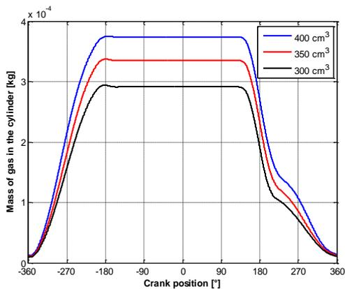
Figure 16. In-cylinder mass of gasses for variation of cubic capacity.
