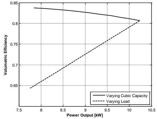
Figure 21. Volumetric efficiency by indicated power.
