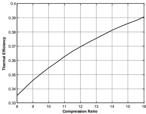
Figure 7. Influence of the compression ratio on the thermal efficiency.
