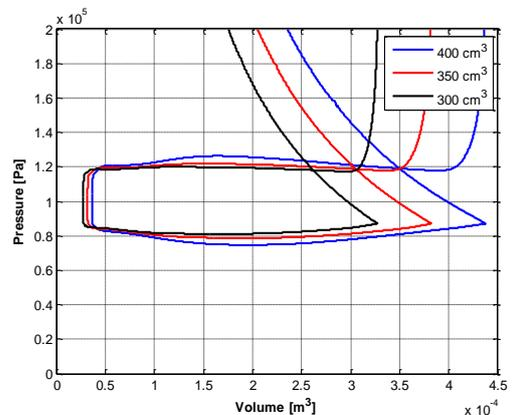
Figure 18. Detail of the open processes on the P-V diagram for variation cubic capacity
