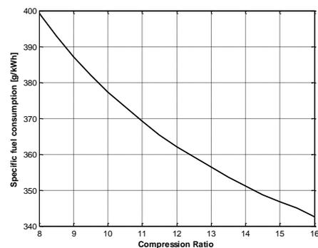
Figure 10. Influence of the compression ratio on the specific fuel consumption
