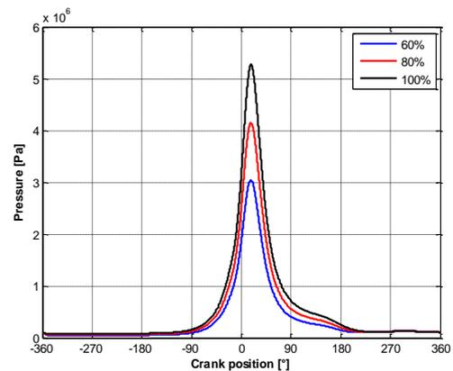
Figure 13. In-cylinder pressure for variation of load
