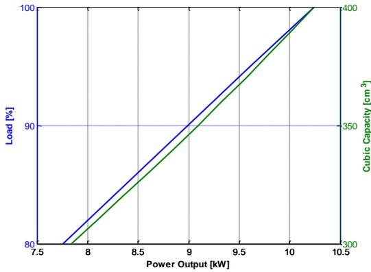
Figure 19. Comparison of the developed power by varying each load and cubic capacity.
