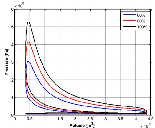
Figure 14. Pressure-volume diagram for variation of load
