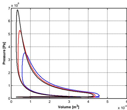
Figure 11. Pressure-volume diagram for variation of compression ratio
