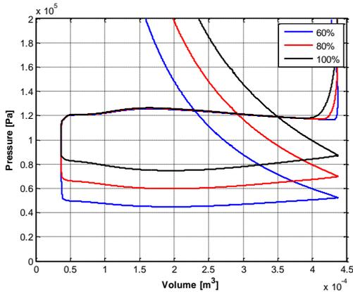
Figure 15. Detail of the open processes on the P-V diagram for variation of load
