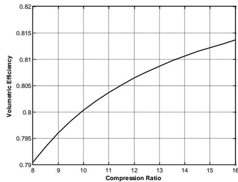
Figure 9. Influence of the compression ratio on the volumetric efficiency
