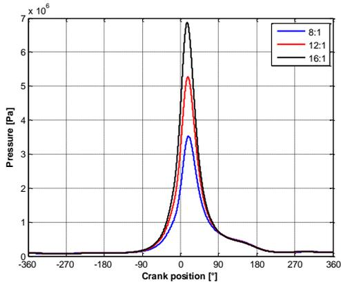
Figure 6. In-cylinder pressure
