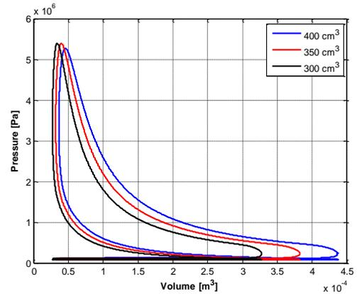
Figure 17. Pressure-volume diagram for variation of cubic capacity.
