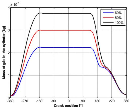
Figure 12. In-cylinder mass of gasses for variation of load.
